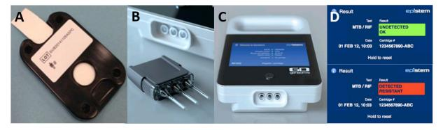
*Notes*: Paper lysis device v2.0 for rapid sample preparation (A); test cartridge with three reaction tubes for MTBC, RIF and control (B); Genedrive<sup>®</sup> instrument (C); test data output with a negative result (upper) and positive result (lower) (D). *Source:* Images reproduced with permission from Epistem.
