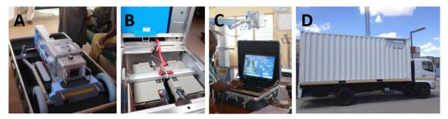
*Notes*: Collapsed DCXR unit in protective flight case (A); battery pack powering the DXR unit (B); CAD4TB system in operation (C); highlights the work in Zimbabwe with the incorporation of the EasyPortable DCXR as a mobile unit housed in a shipping container mounted on a truck (D). *Source:* Images reproduced with permission from Delft Imaging Systems.
