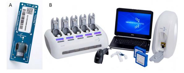
*Notes:* Both PCR amplification and microarray hybridization are performed in the VereMTB<sup>TM</sup> Detection chip. The VerePLEX<sup>TM</sup> Biosystem includes a five-unit processing station for the on-chip PCR and the subsequent hybridization and washing of the chip. For analysis each chip is manually inserted into the reader that interrogates the array (right). *Source:* Image reproduced with permission from Veredus Laboratories.
