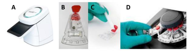
*Notes:* GenePOC Diagnostics automated test device (A); reaction cartridge and sample loading (B, C); loading of the test cartridge (D). *Source:* Images reproduced with permission of GenePOC Diagnostics.
