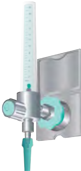
Illustration 10: Oxygen outlet: conditioning and regulation using a flowmeter
