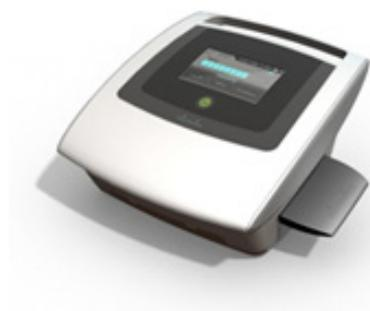
The cartridge incorporates probes, primers, enzymes, buffers and controls for sample purification, amplification and detection, and because it is a closed-cartridge system, there is no PCR product cross-contamination. Cartridge design permits storage at ambient temperatures for prolonged periods. All waste is captured in the cartridge for safe disposal.
