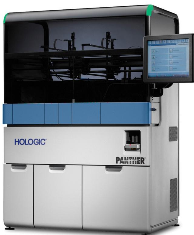
As part of its growing virology offering, the company is developing a quantitative HCV viral load assay, the Aptima® HCV Quant Dx assay for the Panther® System. The Aptima® assay requires three main processing steps, all of which take place in a single tube on the Panther® System: (i) target capture; (ii) target amplification by transcription-mediated amplification (TMA); and (iii) detection of the amplification products (amplicon) by fluorescent-labelled probes (torches).
