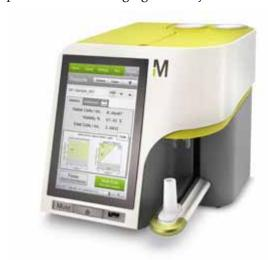
The Muse cell analyser is easy to use. The primary skills required are pipetting and operating the software on the analyser. The Muse requires only 10µL of patient sample. Sample preparation requires two simple dilutions and two 15-minute incubations. The operator loads the CD4/CD4% reagents on the Muse Auto CD4/CD4% system and then follows easy guided menus on the Muse touchscreen. Results, which are displayed in both graphical and statistical formats, are provided within 2–4 minutes.
