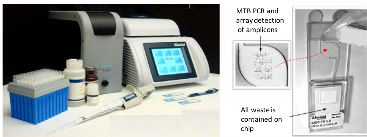
Figure 12. Akonni TruDx ® 2000 platform with TruTip ® extraction pipette, TruArray ® processor and TruArray ® scanner (left); TruArray ® test, microfluidic valve-less design for simultaneous on-slide PCR and microarray hybridization in a closed format (right)
