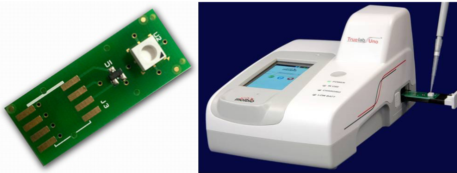
Figure 8. Truenat™ micro PCR chip (left) and Truelab™ Uno Real Time micro PCR Analyzer (right)
