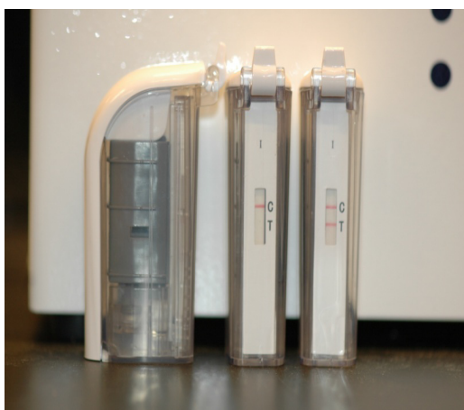
Figure 11. Ustar encased CPA amplicon detection cassette.
