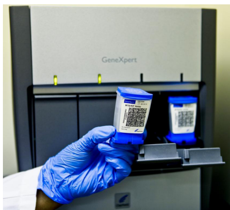
Figure 3. The Xpert® MTB/RIF test cartridge and the GeneXpert® IV instrument by Cepheid
