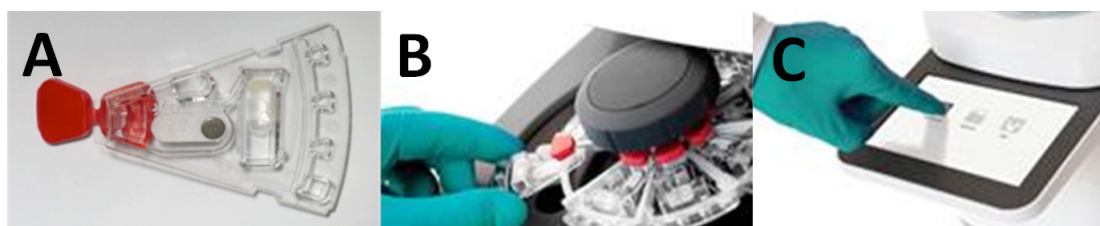
Figure 29. GenePOC test cartridge and instrument: A: GenePOC test cartridge; B: GenePOC instrument (carousel); C: touchscreen interface
