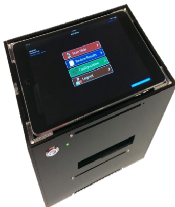
Figure 11. CellScope TB Microscope with a tablet on top for image capture, analysis and viewing
