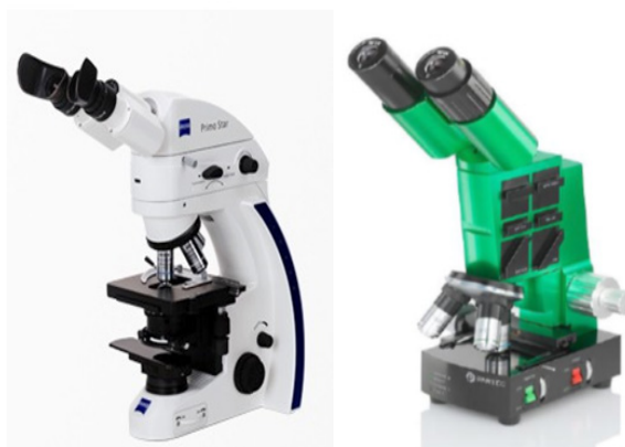
Figure 7. Examples of LED-FM products: Zeiss Primo Star iLED (left); Partec CyScope® (right)
