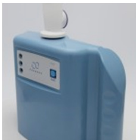
Figure 19. Hand-held Aenose VOC monitor for TB diagnosis produced by the eNose Company
