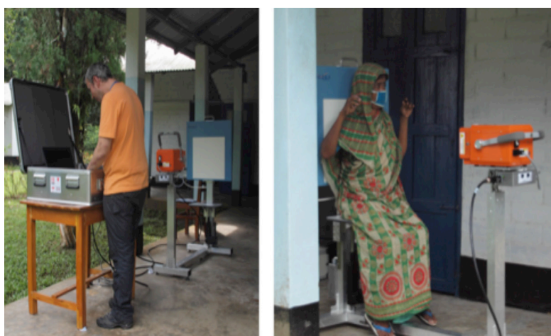
Figure 4. Example of the small size and portability of digital X-ray equipment and its potential for use outside of clinical settings
